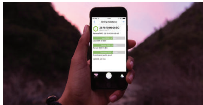
LinqAssist application is available for Android and iOS devices. It requires an external USB dongle to connect MetroLinq device to your phone via Bluetooth. It shows local and remote radio signal levels which is very handy when performing the alignment of your link.
